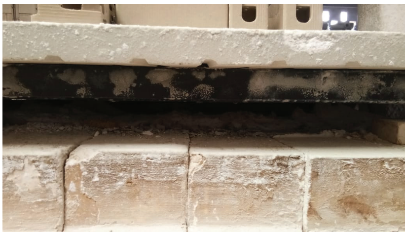
Figure 69: Low thermal mass in Kiln car
