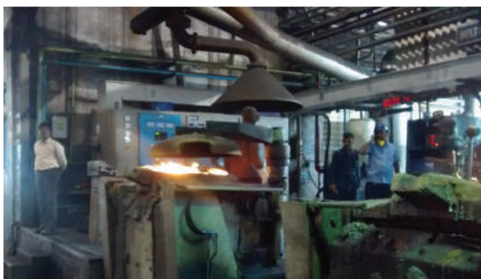
Figure 12: Induction Furnace Lid Mechanism
